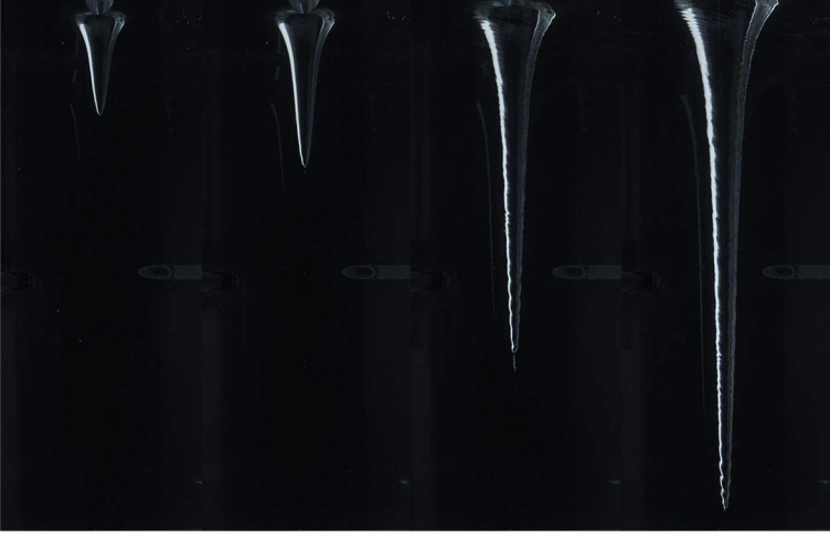
Figure 3.10: Free-surface vortex air core depths H_D for series 5 to 8 with from left to right: H_D = 0.17 m, H_D = 0.26 m, H_D = 0.54 m and H_D = 0.85 m. All air cores are typically funnel shaped.
